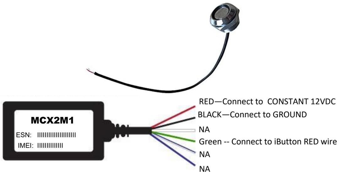
Your iButton receiver will have two wires, a Red and White. Connect the RED wire from the iButton receiver to the GREEN wire on your GPS tracker. Next, connect the WHITE wire from your iButton receiver to a vehicle ground.
