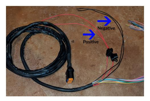
The TitanLTE comes with two POSITIVE and two NEGATIVE wires. This is for redundancy if you wish to connect your
